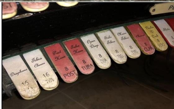
New console bolsters with SAMs. All stop tabs have had the old paper removed and cleaned.
